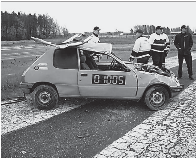
Figure 15. The occupant compartment collapsed while the vehicle rolled over.
