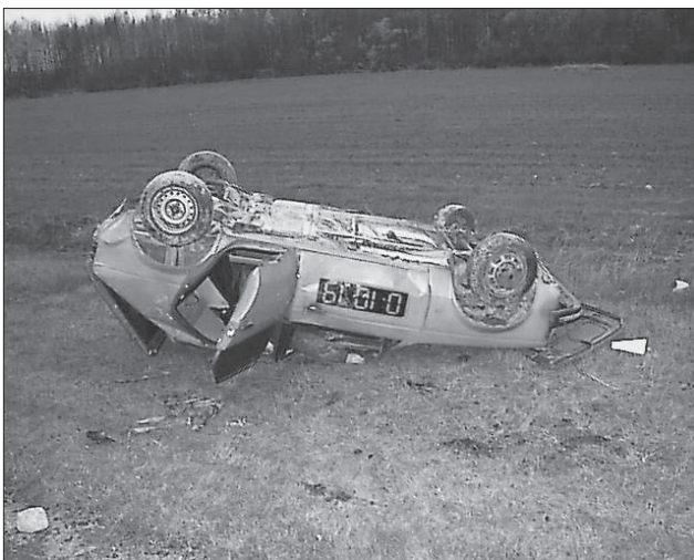
Figure 23. The occupant containment suffered bad damages.
