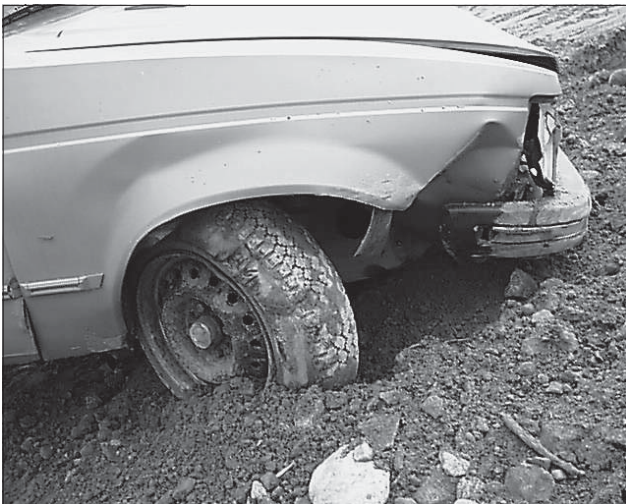
Figure 19. The right front side buckled.
