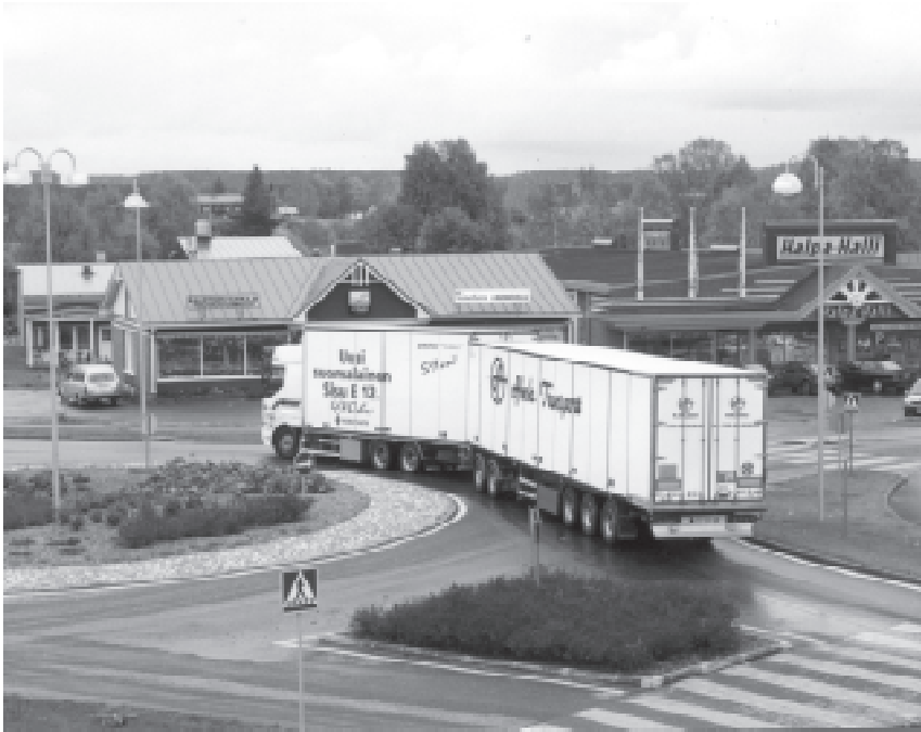
A typical Finnish vehicle combination (Sisu E12); mass 60 tons and length 25.25 metres.
