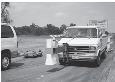
Figure 1. A GPR survey vehicle on road.
