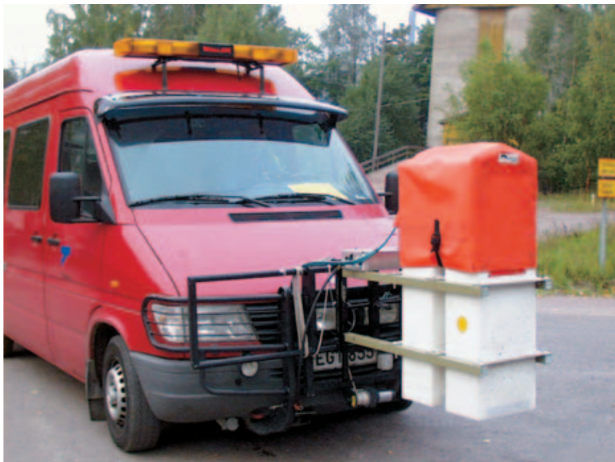
Figure 1. A Finnra GPR van used in asphalt quality control.
