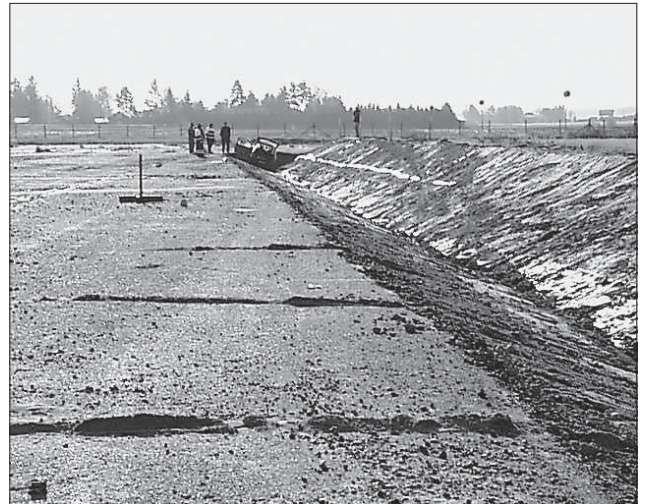
Figure 12. The impact angle was smaller than meant to be. The vehicle exceeded the bottom of the ditch only slightly.
