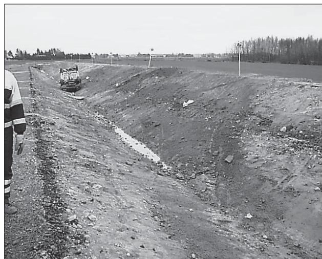
Figure 20. The tyre prints end soon after hitting the back slope.
