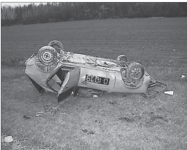
Figure 23. The occupant containment suffered bad damages.
