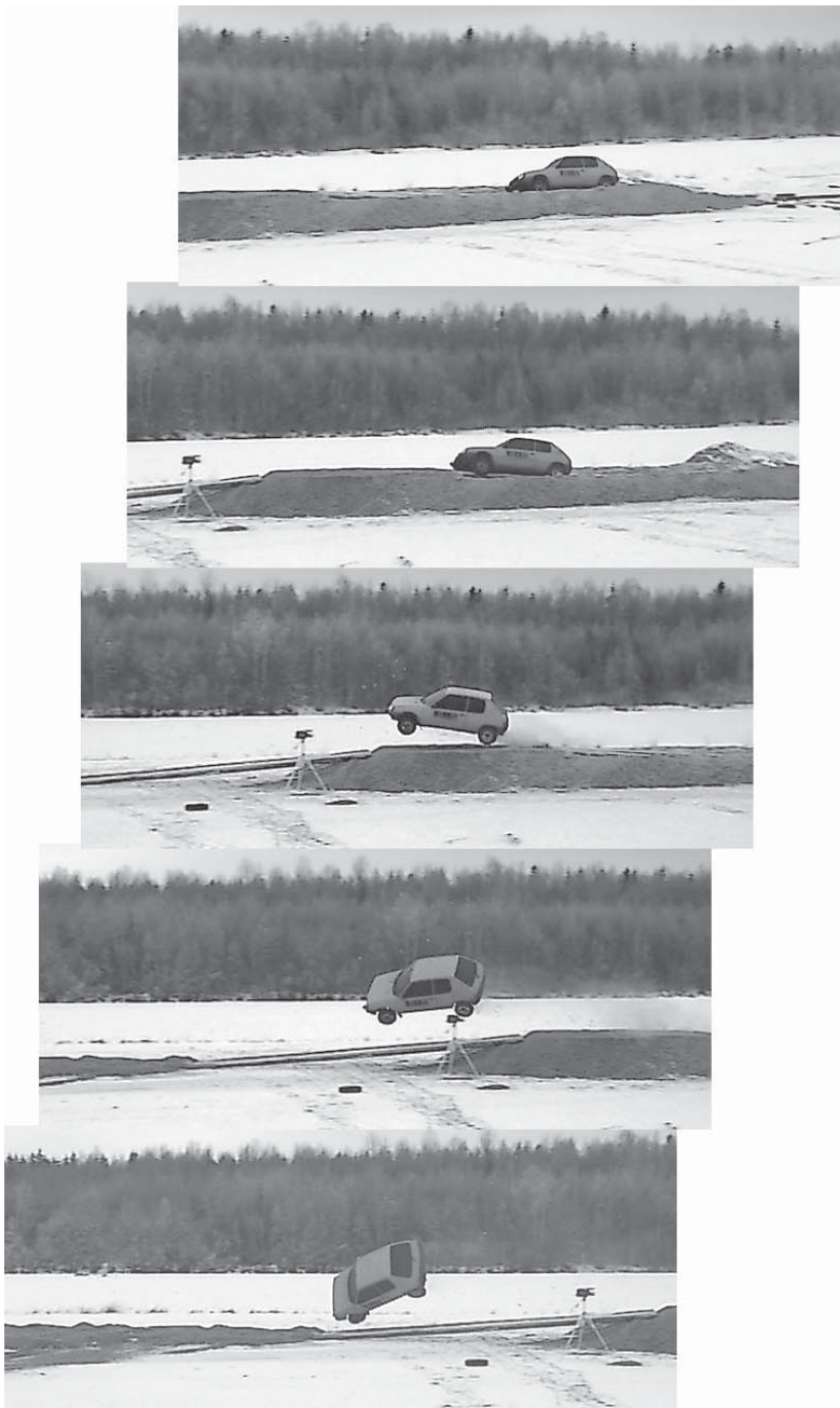
Figure 6. On the third test the vehicle landed the left front corner ahead and rolled over several times.
