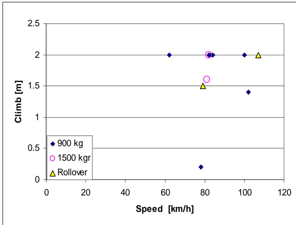
FIGURE 11: The Influence of Vehicle Size and Impact Speed on Climb
