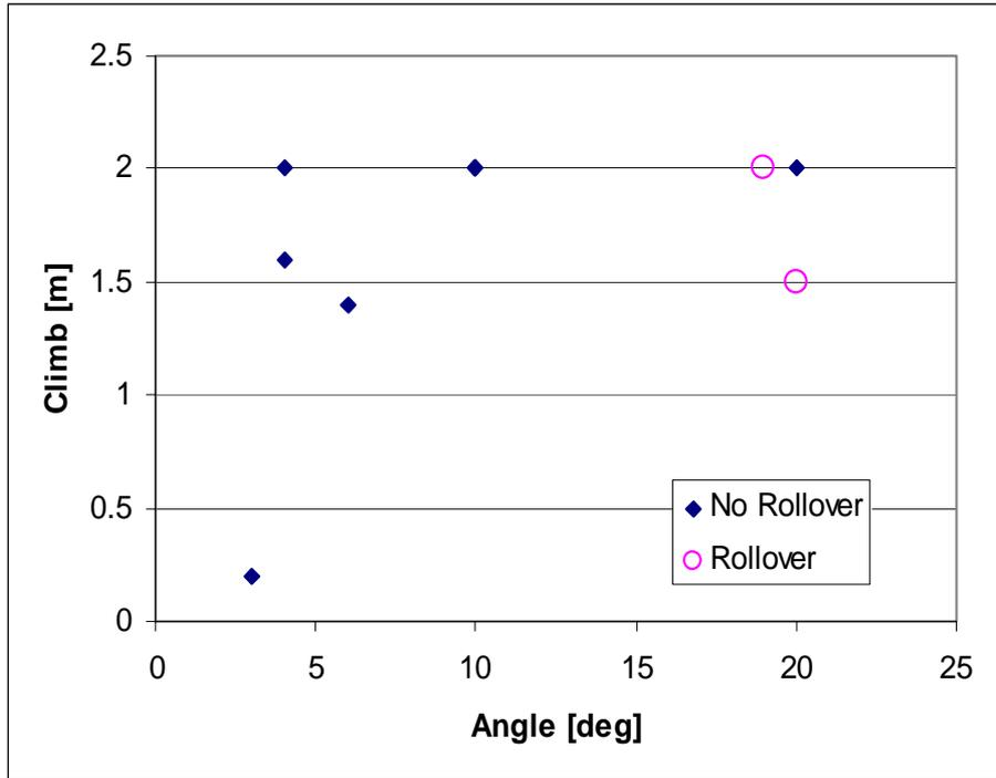
FIGURE 8: Influence of Angle on Vehicle Motion in the Ditch
