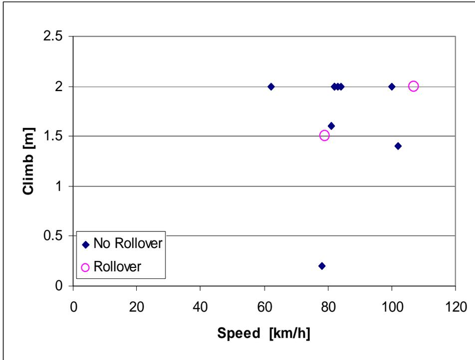
FIGURE 7: Influence of Speed on Vehicle Motion in the Ditch
