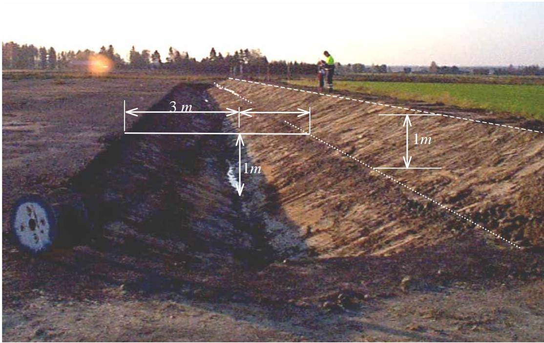
FIGURE 2: Ditch profile for crash testing
