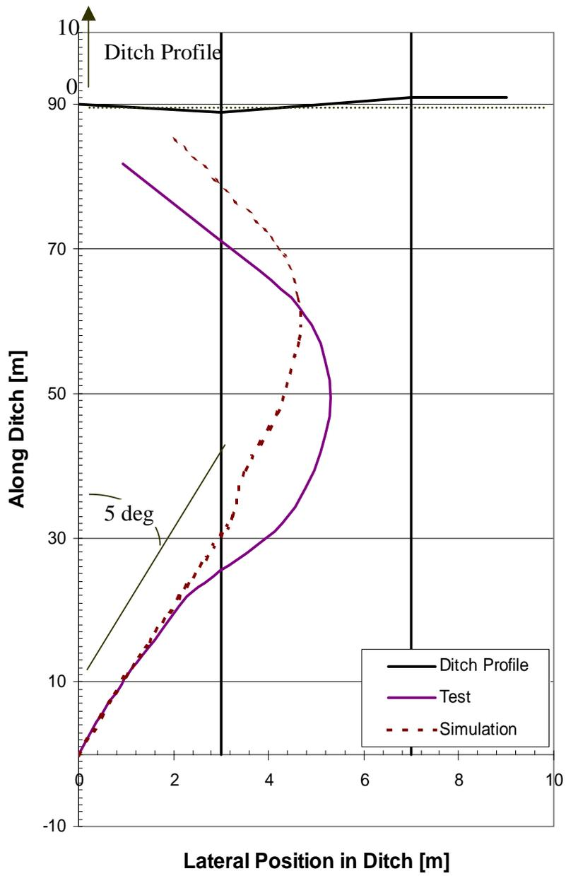
FIGURE 12: Vehicle Path in Test 3 (5 degrees 102 km/h)
