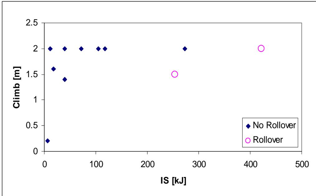
FIGURE 9: Influence of Impact Severity on Vehicle Climb
