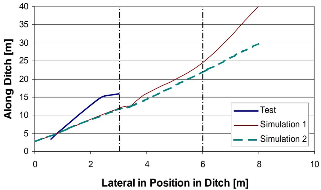
FIGURE 14: Simulation and Test Results in Test 6 - Rollover (20 deg. & 82 km/h)
