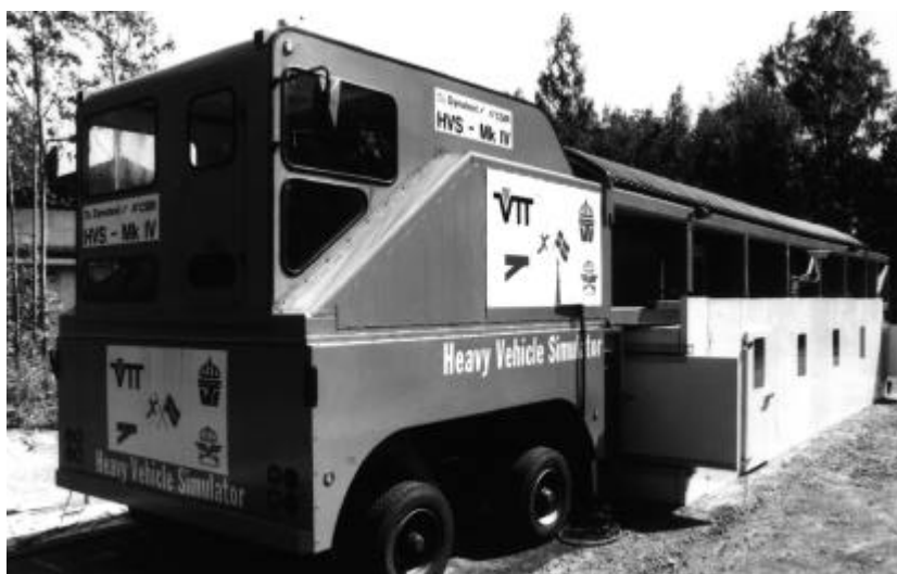
Figure 1. HVS-NORDIC accelerated testing facility.
